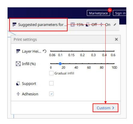
② The parameter **Build Plate Adhesion** → **Build Plate Adhesion Type** needs to be set to "None" when you print the maximum size model.
