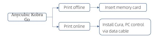
It is suggested to use **Print Offline** mode to minimize the noisy signal via data cable.
