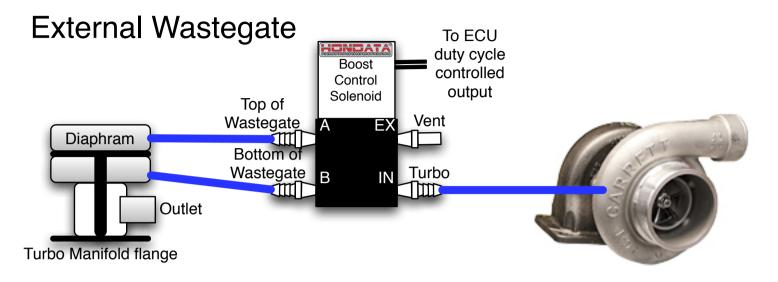
Plumb the port labelled A to the top of the waste gate Plumb the port labelled B to the bottom of the waste gate Plumb the port labelled IN to a source of boost pressure Connect the vent filter to the port labelled EX
