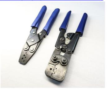
4. With the terminal in the crimper, insert the wire/seal into the terminal. The end of the bare wire should end up even with the part on the terminal that will crimp it. When aligned, crimp
