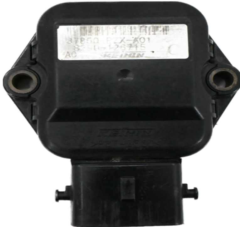
Image 6. TPS Control Module. Part #: 37850-PZX-A01
