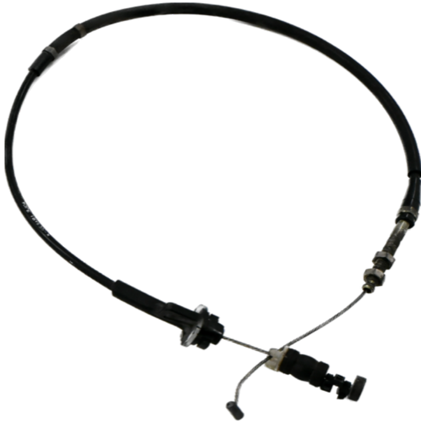
Image 5. Accelerator pedal cable. Part #: 17910-SDB-A03
