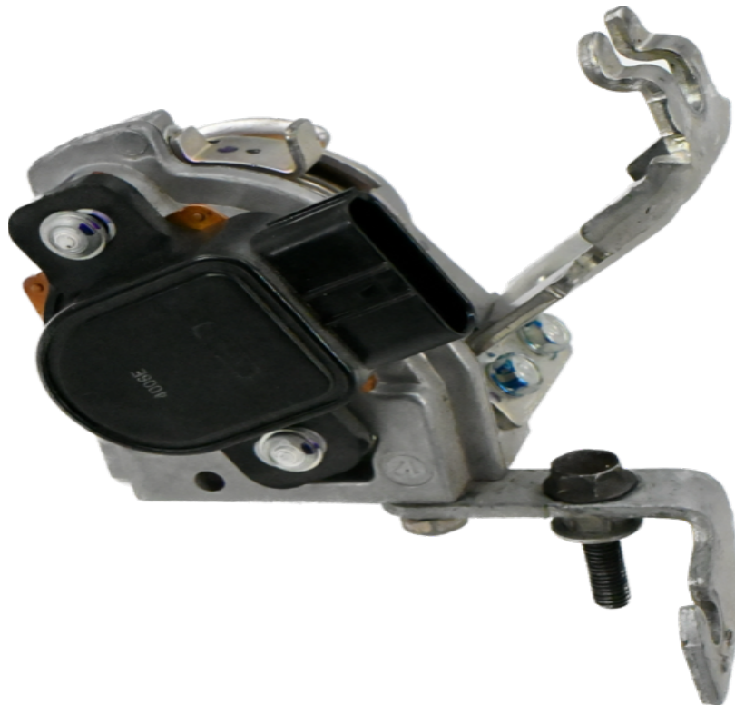
Image 4. Accelerator Pedal Position. Part #: 37971-RCA-A01
