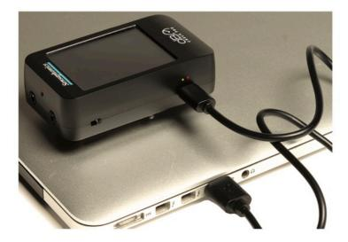
dB Check Pro uses an internal lithium-ion rechargeable battery, which is partially charged when shipped. The battery should be fully charged prior to initial use, as follows:
