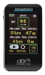
Thank you for purchasing the Sensaphonics dB Check Pro sound level analyzer. Much like a speedometer in a car does for the driver, dB Check Pro gives you the information you need to help you monitor more safely. With dB Check Pro, in-ear monitor (IEM) and headphone users can learn how loud they are listening, in real time, even with earphones inserted.
