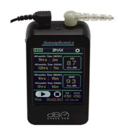
After setup, you're ready to use dB Check Pro. First, use the supplied audio jumper cable to insert the device in-line between the sound source and your IEMs or headphones, using the input/output jacks on the top panel. Note: Either jack can be used for the sound source input or IEM/headphone output. Once connected, turn the Power on. This will take you to the HOME screen.
