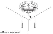
\* Break knockout and put the wire through wire lead on base unit, when exposed wiring.
