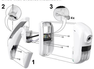
If wall bracket tamper is connected, tamper will automatically be detected by the camera. Tamper will follow recognition settings set in the panel.
