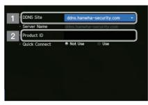
Go to <DDNS> in the recorder <Network> setup menu. 4 Connect to <ddns.hanwha-security.com> and check if the connection status of the registered product is set to <**ON**>.
