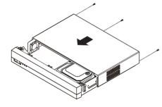
Loosen the screws on the left/right sides and back 2 Connect the SATA/power cable of the HDD to the connector on the motherboard.
