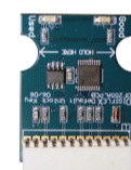
P/N - CM255B Panel Default Unlock Key Will reset Installer PIN and RAS PIN on Solution 6000 panels. F.01U.271.514
