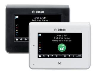
The keypad is an SDI2 bus compatible device. The keypad features an illuminated touch screen and graphical interface. With an elegant design and low profile, the keypad fits with any modern decor. Each keypad has user adjustable options such as volume and brightness. They have four inputs and one output. The keypad shows system messages for all areas.
