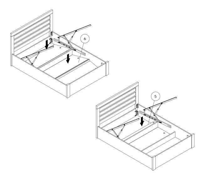
**Step 8**: Attach the bed base to the hydraulic frames using hardware part L. Fix the bolts starting from area 1 and finishing in area 3 – do not fully tighten the bolts yet.
