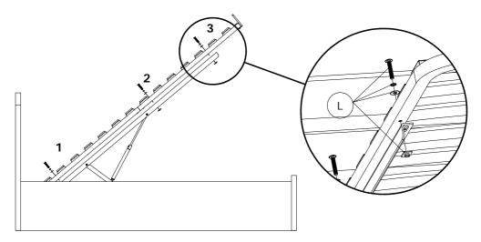
**Step 9**: Adjust the bed base, make sure that the distance to the footboard is approximately 15 mm to above. Tighten all bolts and screws now.
