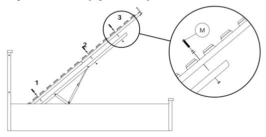
**Step 10**: Adjust the bed base making sure that the distance to the footboard is approximately 15 mm to above. Tighten all bolts and screws now.
