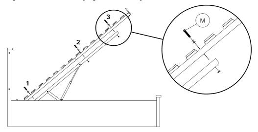
Step 10: Adjust the bed base, make sure that the distance to the footboard is approximately 15 mm to above. Tighten all bolts and screws now.
