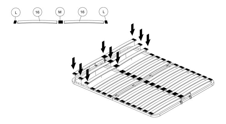
Step 8: Insert the Small Base Panel (8) and Large Base Panels (9).
