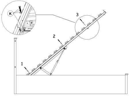
Step 10: Carefully lower the Metal Base using the Base Handle at the Footboard End. A moderate amount of force will be required, if necessary place your mattress on top of the Metal Base to assist with this.
