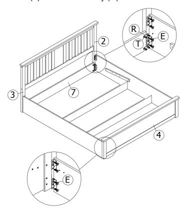
Step 4: Attach the Metal Corner Support (C) to the Footboard (4) and Side Rails using hardware (E & P).
