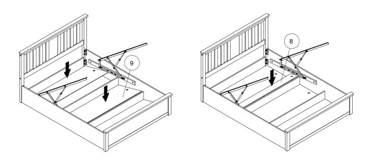
Step 9: Attach the assembled Metal Bed Base to the Hydraulic Base Supports (11 & 12) using hardware (K & P), but don't fully tighten the bolts. Start from headboard, then the middle and finally the footboard.
