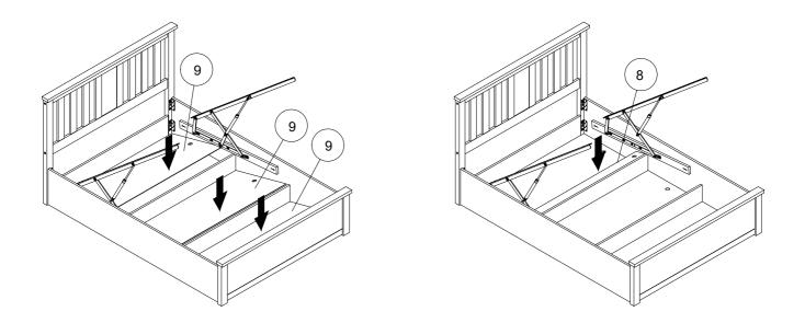
Step 9: Attach the assembled Metal Bed Base to the Hydraulic Base Supports (11 & 12) using hardware (K & P), but don't fully tighten the bolts. Start from headboard,then the middle and finally the footboard.
