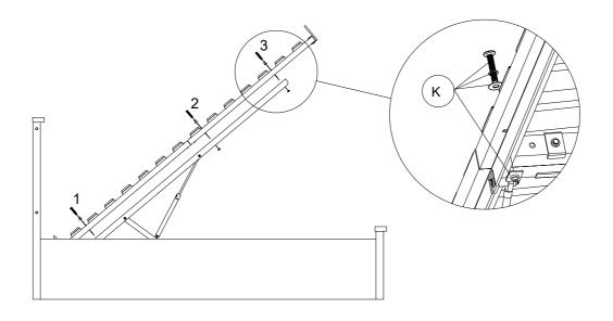
Step 10: Carefully lower the Metal Base using the Base Handle at the Footboard End. A moderate amount of force will be required, if necessary place your mattress on top of the Metal Base to assist with this.
