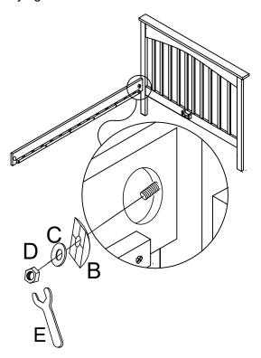
Step 3: Attach the Side Rails to the Footboard by repeating steps 1 and 2. Once the frame is secure, please tighten all 4 ends fully using the Spanner (E).
