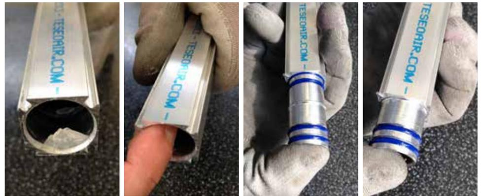
**3 HOW TO CONNECT TWO PIPES WITH A STRAIGHT JOINT**
