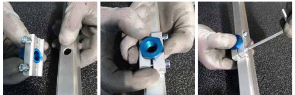
**⚠ WARNING:** After each joint is complete, check you have locked all the screws and you have not damaged the threads by over tightening.
