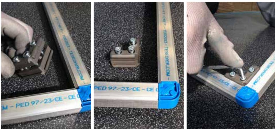
**⚠ WARNING:** After each joint is complete, check you have locked all the screws and you have not damaged the threads by over tightening. The recommended tightening torque for the screws is a minimum of 10 Nm to a maximum of 13.5Nm. In practice, once the screw has come to a stop, make one more ¼ turn.
