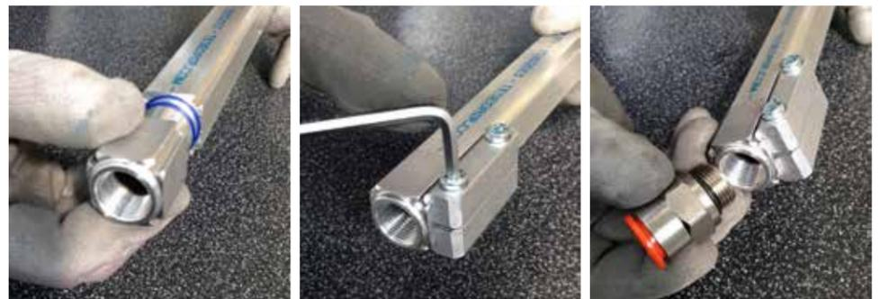
Inserting the threaded terminal
