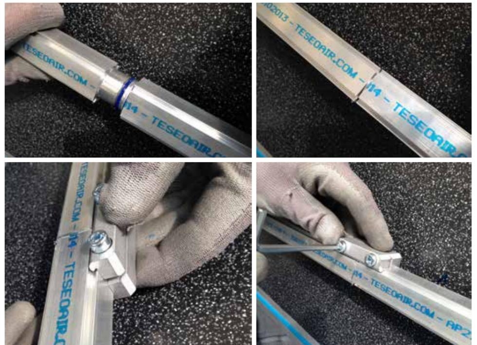
The screws should be tightened with the allen key. The recommended tightening torque for M5 screws is between 9 Nm and 11 Nm. Once the screw has come to a stop, make one more 1/4 turn. **WARNING:** After each joint is complete, check you have locked all the screws and not damaged the threads by over tightening.
