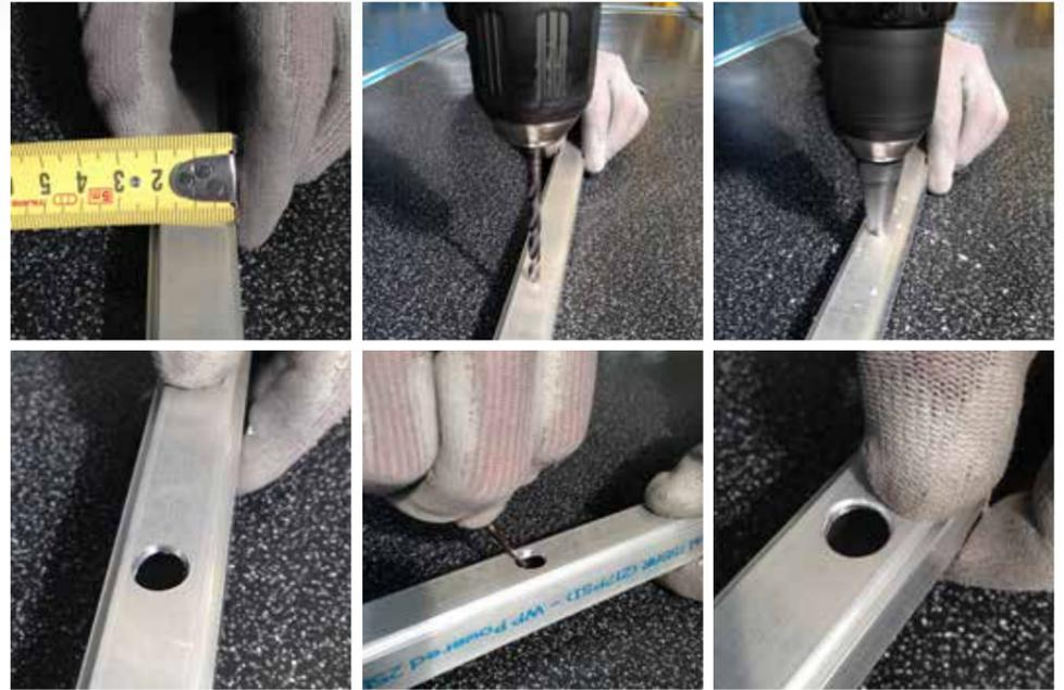
Once done, clean the hole. Attach the outlet plate inserting the clamp in the dovetail grooves and tighten the screws. The recommended tightening torque for the M5 screws is between 10Nm and 13.5Nm. (Once the screw has come to a stop, make one more ¼ turn.)
