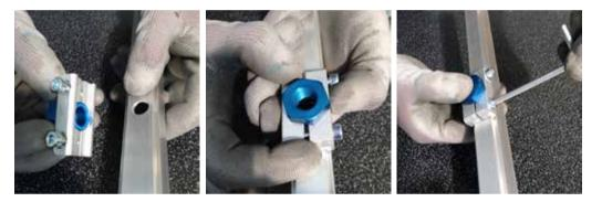
🖄 WARNING: After each joint is complete, check you have locked all the screws and you have not damaged the threads by over tightening.
