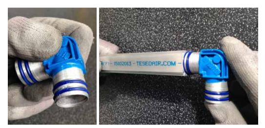
After the the two sections of pipe have been connected with the "L" joint, insert the provided "L" clamping bracket in the dovetails grooves and tighten the screws. The recommended tightening torque for M5 screws is between 10Nm and 13.5Nm. (Once the screw has come to a stop, make one more 1/4 turn.)
