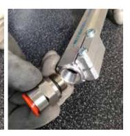
Inserting the threaded terminal
