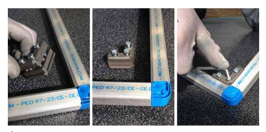
N WARNING: After each joint is complete, check you have locked all the screws and you have not damaged the threads by over tightening. The recommended tightening torque for the screws is a minimum of 10 Nm to a maximum of 13.5Nm. In practice, once the screw has come to a stop, make one more 1/4 turn
