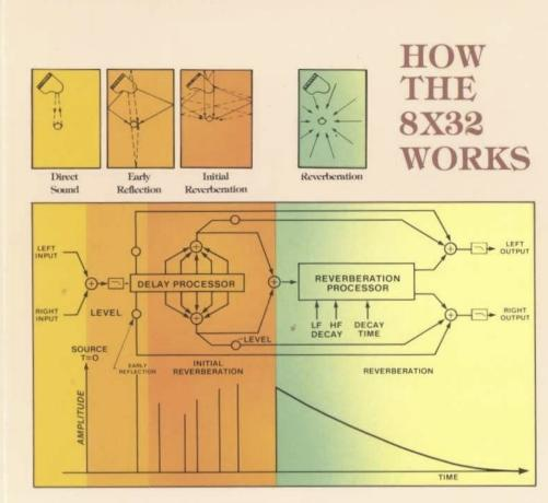
In a naturally reverberant space, direct sound impulses reflect off boundary walls and then quickly diffuse throughout the space. The 8X32 simulates this effect with three independently-controlled processing stages. When direct sound is fed into the unit, early reflections are first generated, to lend body to the sound and help define the size of the
