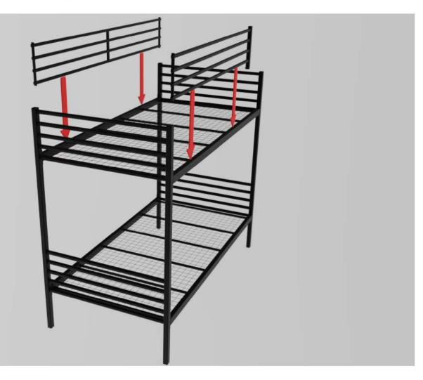
Attach front and back safety rails to frame by the relevant bolt holes.
