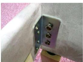
Standing the headboard against a wall and facing the headboard attach the left-hand side rail on to the affixed brackets as picture.
