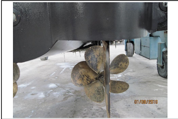
Starboard Prop & Rudder
