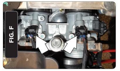
Unplug the stock wiring harness from both of the fuel injectors as shown in Figure F.
