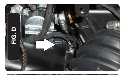
Unplug the electrical connector for the throttle body servo on the left side of the throttle bodies as shown in Figure D.
