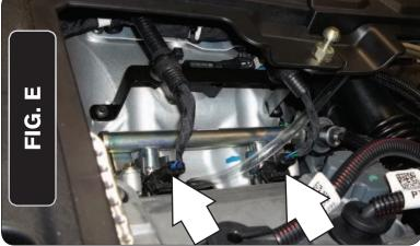
Unplug the stock wiring harness from each of the fuel injectors (Fig. E).
