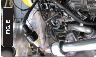
Plug the Pro tuner wiring harness in-line of the TPS and the stock wiring harness (Fig. E).
