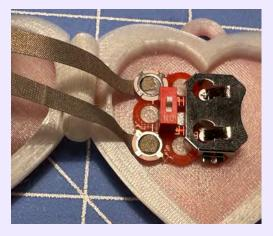
Insert 3v battery into the holder, then gently press/ rock the battery holder onto the pegs over the etape, ensuring a good connection
