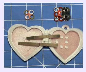
Line up your parts as shown and cut your e-tape strips, then peel the backing and apply to pegs, making sure they do not touch each other
