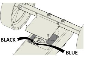
Install the second battery with the terminals facing in towards the handle. For Traps fitted with the large battery tray this step is not necessary as the ring terminals provided on the cable be connected to the appropriate existing battery connector
