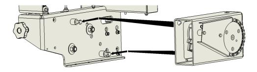
The two main fixing bolts can now be fully tightened, followed by the front casting plate nut. Refit the front and rear plastic caps, taking care not to trap the electrical wiring in the process.
