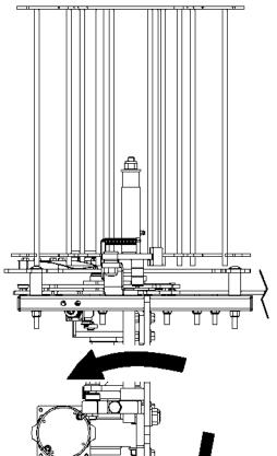
Loosen the locknut on the side opposite to the side you wish the trap to tilt towards, back off the bolt and the trap should begin to tilt away from you.
