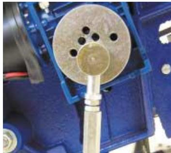
By placing the crank bolt in a different hole on the disc the angle of elevation can be adjusted. The further out the hole from the centre on the disc, the more up and down movement is achieved.
