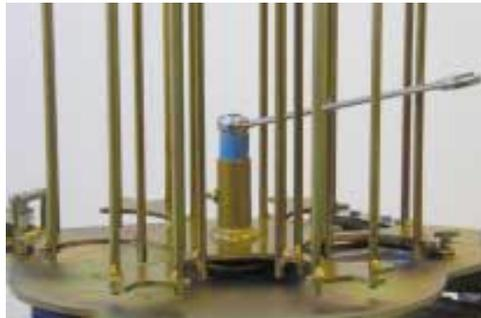
**If your trap was delivered without its mainspring fitted, now is the time to fit it.** The Arm(s) can now be moved by hand until they stick directly out of the front of the trap away from the operator. The mainspring would now normally be at its shortest length and can therefore be fitted to the machine. See following photo.
