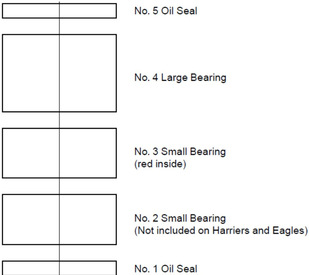
**Note:** — Install the seals and bearings with markings on the upper face.
