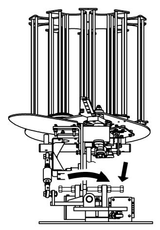
Loosen the locknut on the side that you wish the trap to tilt towards, back off the bolt and the trap should begin to tilt towards from you.
