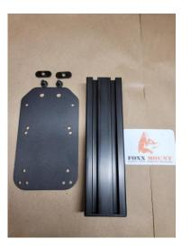
Each mount has a Horizontal Assembly. The assembly consists of the appropriate stick or throttle plate, a 7"\* horizontal beam, 2x(1/4-20 x 3/8" bolts), 2x(1/4-20 slide nuts), as well as 2 anchor assemblies used to connect the Horizontal and Vertical Assembly
