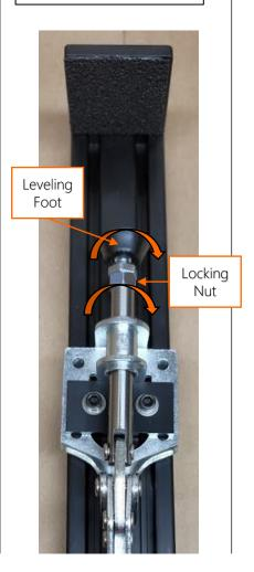
For larger adjustments, use the included Hex Key to loosen the two screws holding the Toggle Clamp, and shift up and down as needed. It should only take a turn or so to loosen. Tighten firmly when done.
