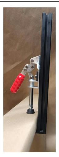
Take an Anchor Assembly and loosen the nut on it such that only a few threads are engaged. Then slide it into the left slot as shown.
