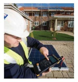
PV installation test IEC 62446 describes a variety of techniques for shorting a string during testing and taking measurements using clip-on ammeters.
