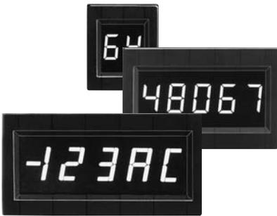
The modules possess a 7 segment LED matrix. The numeric versions display the figures 0 to 9, and the hexadecimal versions the characters A to F in addition. For applications with longer data lines between the display and the control, pin compatible modules with Schmitt trigger inputs are available; the Schmitt trigger versions are also available with inverted BCD/binary data inputs.
