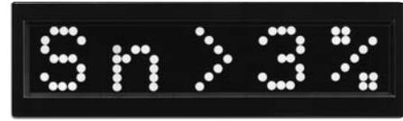
The display modules D72-422 are equipped with a 5x7 LED dot matrix and can display small and capital letters, numbers and special characters. The Schmitt trigger characteristic on all data inputs grants high noise immunity, even in cases of long data lines between control and display.
