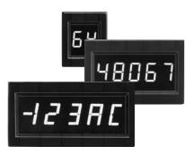
The modules possess a 7 segment LED matrix. The numeric versions display the figures 0 to 9, and the hexadecimal versions the characters A to F in addition. For applications with longer data lines between the display and the control, pin compatible modules with Schmitt trigger inputs are available; the Schmitt trigger versions are also available with inverted BCD/binary data inputs.
