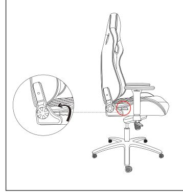
Pull the lever FULLY and lean back slowly until desired angle is achieved, then slowly return the lever to its starting position Ensure the lever locks back in place.
