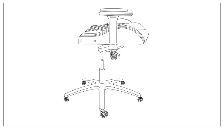
**STEP 7:** Using Adjusters to attach Seat Cushion, align the adjusters over the pre-drilled holes underneath the seat cushion with M8x25mm bolts, tighten all the bolts with the wrench.
