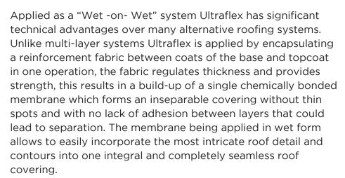
Ultraflex is cold applied, moisture curing and rain resistant instantly after application.
