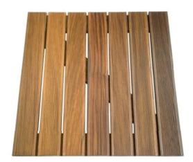
Pre-assembled 500x500 mm, 30 mm thick deck tiles in Ipè wood, each made up of seven 15x67x500 mm boards, to create an anti-slip flooring surface, and three 15x67x500 mm battens for the substructure, positioned in a "Z" formation.
