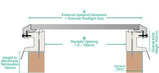
Opening / Ventilated rooflight on structural, insulated builders upstand
