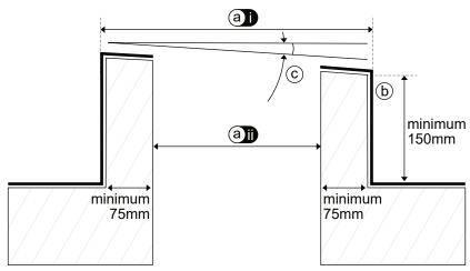
(a) Finished insulated and weathered upstand dimensions:
