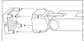
5 Check green LED lights up when power is turned on. If not, remove transparent cover and press yellow test button, LED should flash amber
