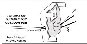
3 Wire into green terminal. Once wired, connect green terminal strip into mounting plate.
