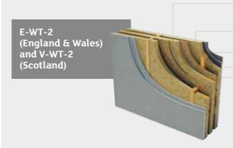
Wall width: 240mm (min) between inner faces of wall linings. 50mm (min) cavity (gap between wall panels) 68mm (min) between stud frames
