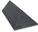
Natural Spanish slates, bonded to a Glass Reinforced Polyester (GRP) substrate, with aluminium rivets for secondary mechanical fixing. For use as a preformed angular dry-fix hip or ridge tile. Fixing holes pre-drilled and fixings supplied.
