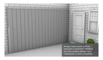
Depending on your installation, you may want to finish off the edges using one of the Trims Cladco can provide to give you a lasting professional look. There are a range of Trims available in all colours to complement your Cladding Boards, which can be secured to your installation by glue, using an exterior grade high elastic glue.
