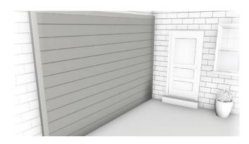
Depending on your installation, you may want to finish off the edges using one of the Trims we can provide to give you a lasting professional look. There are a range of Trims available in all colours to complement your Cladding Boards and these can be secured to your installation by gluing them in place using an exterior grade high elastic glue.
