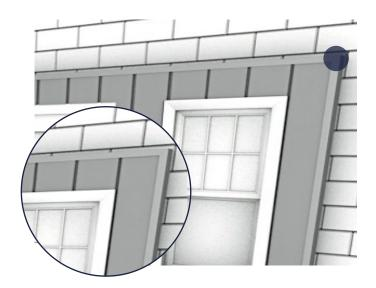
Once the Corner Trim is cut to size, you can use Sumogrip adhesive along one or both sides of the Corner Trim to attach to the edge of the Cladding.
