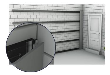
Secure the Boards using a screw at least 30mm in length, ensuring that the Board is fastened securely on each Batten that it touches. Secure these fixings by hand, as it is important not to over-tighten the screws and risk splitting the Board.
