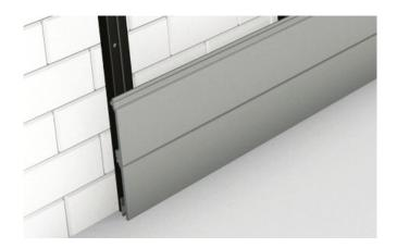
Slot the second Board onto the irst and repeat the fixing process ensuring that the second Board is fitted securely in place on each Batten. Repeat this process with each Board until you reach the required height.
