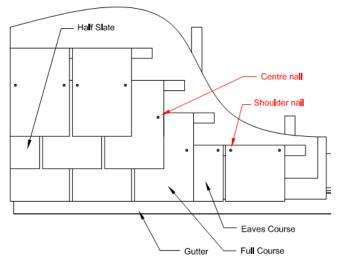
Figure 2 – Fixing the IKO Slate
