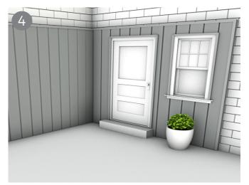
To allow for expansion you may wish to only glue the top edge. Once installed, you can then cut and place the second piece of trim along the edge until you have the desired finished look.
