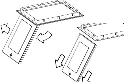
**3.** Trim out a suitable opening (562 x 726mm minimum). Locate frame into position pushing tightly against the ceiling to form seal.
