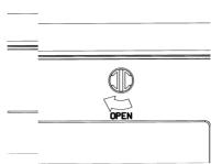
**2.** Swing the door open as far as it will go and then slide side ways slightly to disengage one side of the hinge then remove the door
