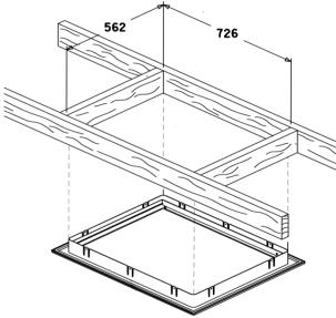
**4.** Screw through the fixing points in ten places as shown. Note Suitable packing pieces may be required if the opening is over size, to prevent the distortion of the frame.
