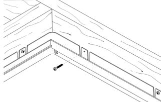
**5.** Finally replace the door into the frame ensuring both hinge lugs are correctly located. Secure door by turning catch anticlockwise. This can be done using a pole with the supplied pole end.
