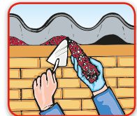
Sealing of corrugated roofs
