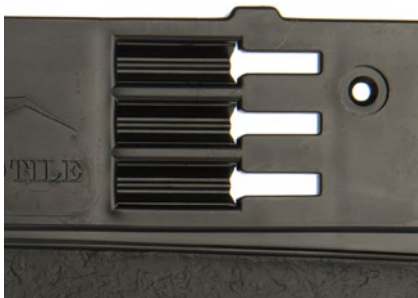
Ensure that you clip the tiles into the right slots depending on the batten gauge used.
