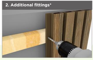
2. Then fix the same cladding plank through the recessed screw groove on the lap edge using a 25mm long plain fixing screw. \* see note at end
