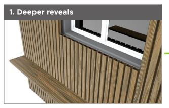
1. For deeper window reveals Edge Boards can be cut to length and to a suitable width so that it finishes flush with the front of the cladding planks.
