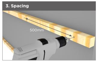
3. The spacing between anchors should be no more than 500mm.
