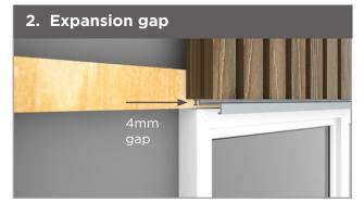
2. Leave a 4mm expansion gap between the bottom of the cladding plank and the drip trim
