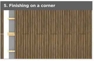
5. When finishing on a corner, cut the last cladding plank to suitable width and fix to a joist using a 35mm long colour head screw through the low valley of the cladding profile.
