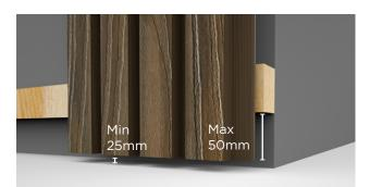
**\*NOTE:** Locate the first joist to ensure a clearance of at least 25mm can be left between the bottom of the cladding plank and the ground surface. The cladding plank should not overhang the bottom joist unsupported by more than 50mm
