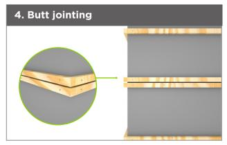
4. When butt jointing two lengths of cladding (runs over 2700mm), it is important to install double joists so that each board is secured to an independent joist.
