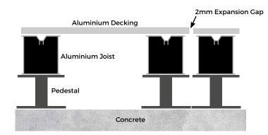
Where two Boards will meet end-to-end, a row of two Joists will need to be in place to support the Boards. Adjust the height of each pedestal to allow for a drainage gradient (12.5mm fall per metre) and secure them into place on the concrete base.
