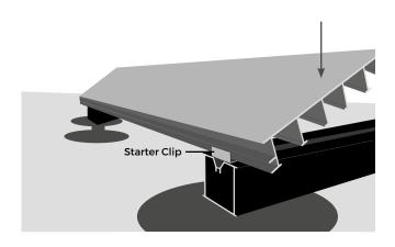
Install the first Decking Board to the Starter Clips, laying the Aluminium Boards perpendicular to the Joists. Where two Boards meet end-toend, allow for a 2mm expansion gap and support over a pedestal. If including an overhang, this should be no more than 30mm.
