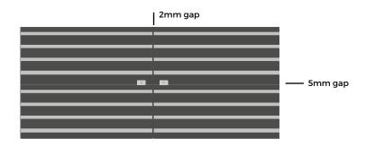
Fix Stainless Steel Clips to the first Board and secure the Clips into place over each Joist underneath using 30mm Screws. We recommend 7 Clips per 3.6-metre Board. Once all Clips are secure, place the next Board into the Clips, leaving a 5mm expansion gap between Board edges.
