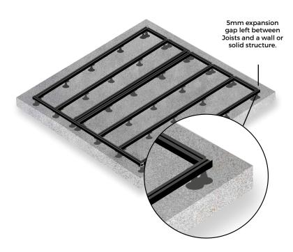
Once all pedestals are secured into the concrete, fix Aluminium Joists onto the pedestals. Where two Joists meet end-to-end, a 2mm expansion gap should be left between ends and supported over a pedestal. A 5mm expansion gap should be left between a wall, or a solid structure, and the Joist.
