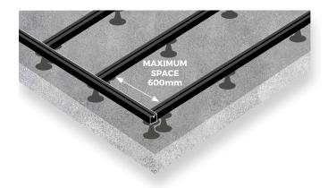
Aluminium Joists should be supported by decking pedestals (not supplied) to create a ventilation gap and a slope for drainage. Begin your installation by marking out pedestal positions across the concrete base, placed at a maximum of 600mm apart from centre to centre. Ensure a pedestal is positioned where two Joists meet end-to-end.
