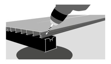
**7** Continue installing Boards Into the Stainless Steel Clips, leaving a 5mm expansion gap between parallel Boards. To secure the last Board, screw through the side of the Board and into the Joist. It is recommended to pre-drill through the Decking Board 1-2mm wider than the Screw.
